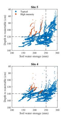
**Figure 7.** Soil water storage vs. water table level at sites 4 and 5. The red colour distinguishes events with high hourly rainfall intensity, defined as  $I_{\text{peak}} > 15$  mm, consistent with Fig. 5. The dashed black lines correspond to values of water level and soil water storage discussed in the text. Soil water storage is measured for the top 60 cm at the Automatic Weather Station.
