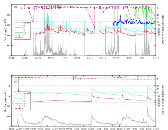
**Figure 6.** Time series of discharge (grey lines) and groundwater levels at sites 4, 5, 3, 32, 2 and 1; manually read sites are shown with dashed lines and diamonds at measurement points. Levels above zero at sites 1 and 2 occur as the soils are highly pugged in the riparian zone and water pooled on the surface in places, leading to slightly positive water levels being measured, at site 2 in particular.
