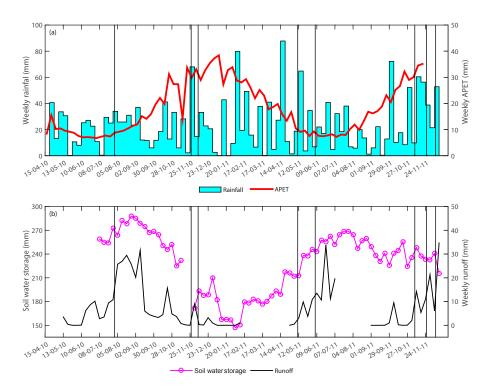
**Figure 3. (a)** Weekly rainfall and APET (areal potential evapotranspiration) time series, **(b)** soil water storage in the top 60 cm of the soil profile and weekly runoff time series for the flume at the catchment outlet. The rainfall, areal potential evapotranspiration and volumetric soil moisture used to calculate soil moisture storage were all recorded at the AWS (automatic weather station) (Fig. 1). The vertical bars show the timing of events in Fig. 4.
