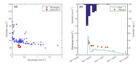
Figure 10. (a) Discharge vs.  $Cl^-$  concentration for all events. The red colour identifies samples from the event on 8 November 2011. (b) Time series of rainfall, runoff and  $Cl^-$  concentration for the event on 8 November 2011.
