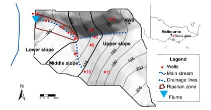
**Figure 2.** The study site location within Australia and a hill shaded DEM, topography and sampling site locations at RBF. In this figure the black circles show shallow groundwater sites, the red circle shows the soil moisture site and the blue triangle demonstrates the catchment flume.
