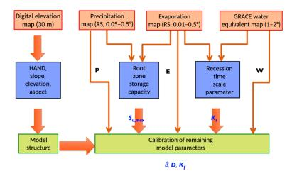
Figure 1. Flow diagram for prediction in ungauged basins.
