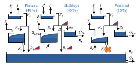
Figure 2. Example of a structure for a semi-distributed model consisting of three hydrologically distinct functional units based on the respective areal proportions of three landscape classes as derived from a digital elevation model, connected by a common groundwater system (after Gharari et al., 2014).
